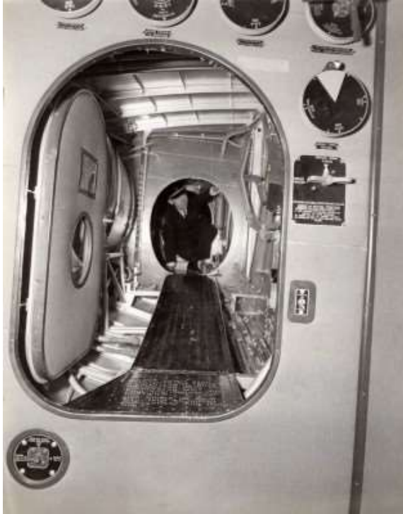
B-314 wing catwalk, allowing access to the engines during flight.
