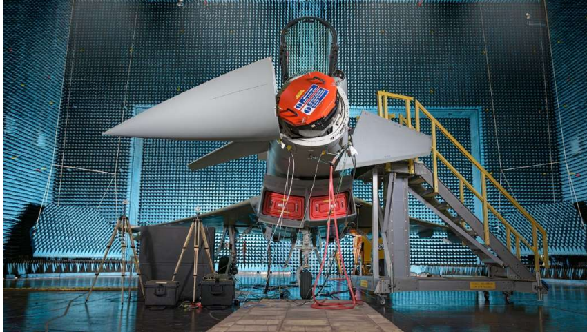
Typhoon with the ECRS radar before first flight (Picture: BAE Systems).
