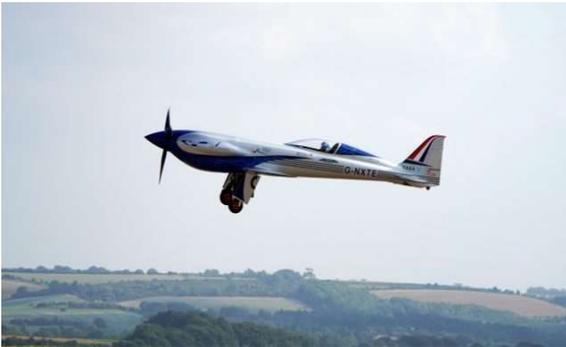
Rolls-Royce's Spirit of Innovation has reached a top speed of 555.9km/h (345.4mph) over 3km, beating the existing record by 213.04 km/h (132mph) on 16 November 2021, according to Rolls-Royce. The aircraft is powered by a 400kW (500+hp) all-electric power train with what Rolls-Royce claims is the most power-dense battery pack ever assembled for an aircraft.
